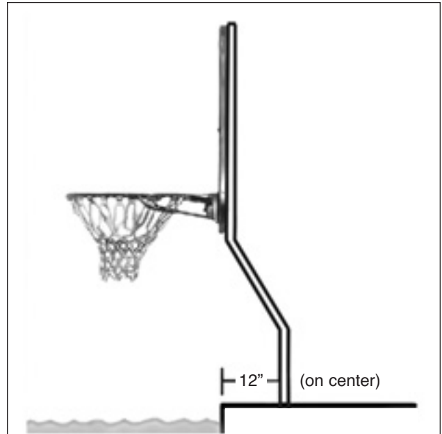
Fig. 16 Anchor Placement - Side View
