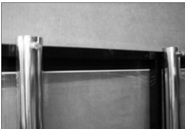
Fig. 22 Support Poles Affixed to Threaded Insert Nuts
